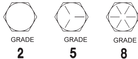
BOLT HEAD GRADE MARKING
